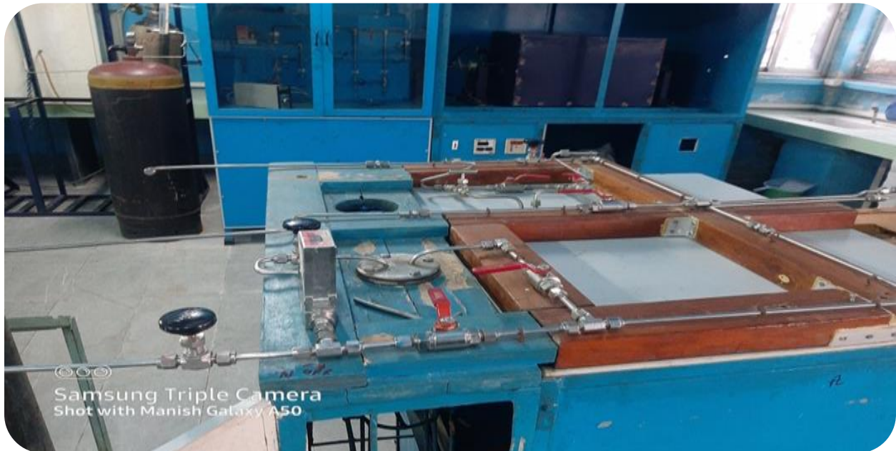
Fig:- Gas sources, gas line and bubblers
