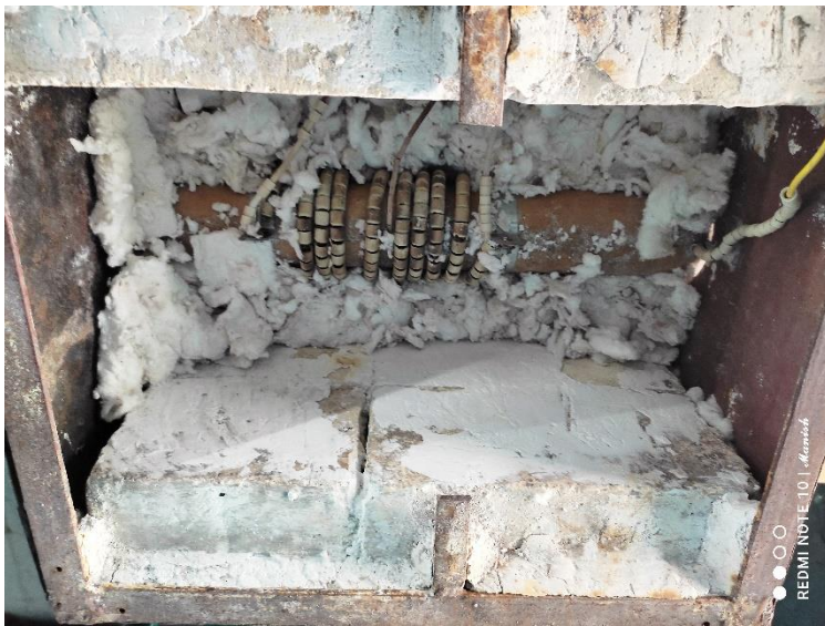
Fig:Single Zone Furnance With Heater coil assmbly and Pack with Silica wool
